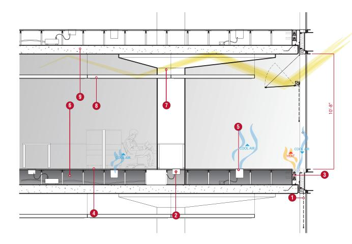
**6. H.V.A.C. COOLING:** Typical floors shall be cooled by a down discharge VAV compartmental unit; each unit shall be fitted with VFD for volume control. Supply air from the under floor plenum shall be released into the occupied space by means of manual and automatic VAV in floor terminals.
