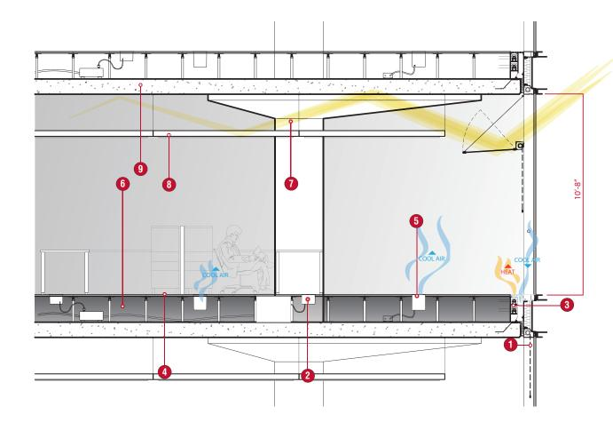
**1. WINDOW SHADING:** Interior roller blinds at all glazed walls. Exterior horizontal aluminum fin type sun shading at the south facing façades. Exterior vertical sun shading at the west façade.
