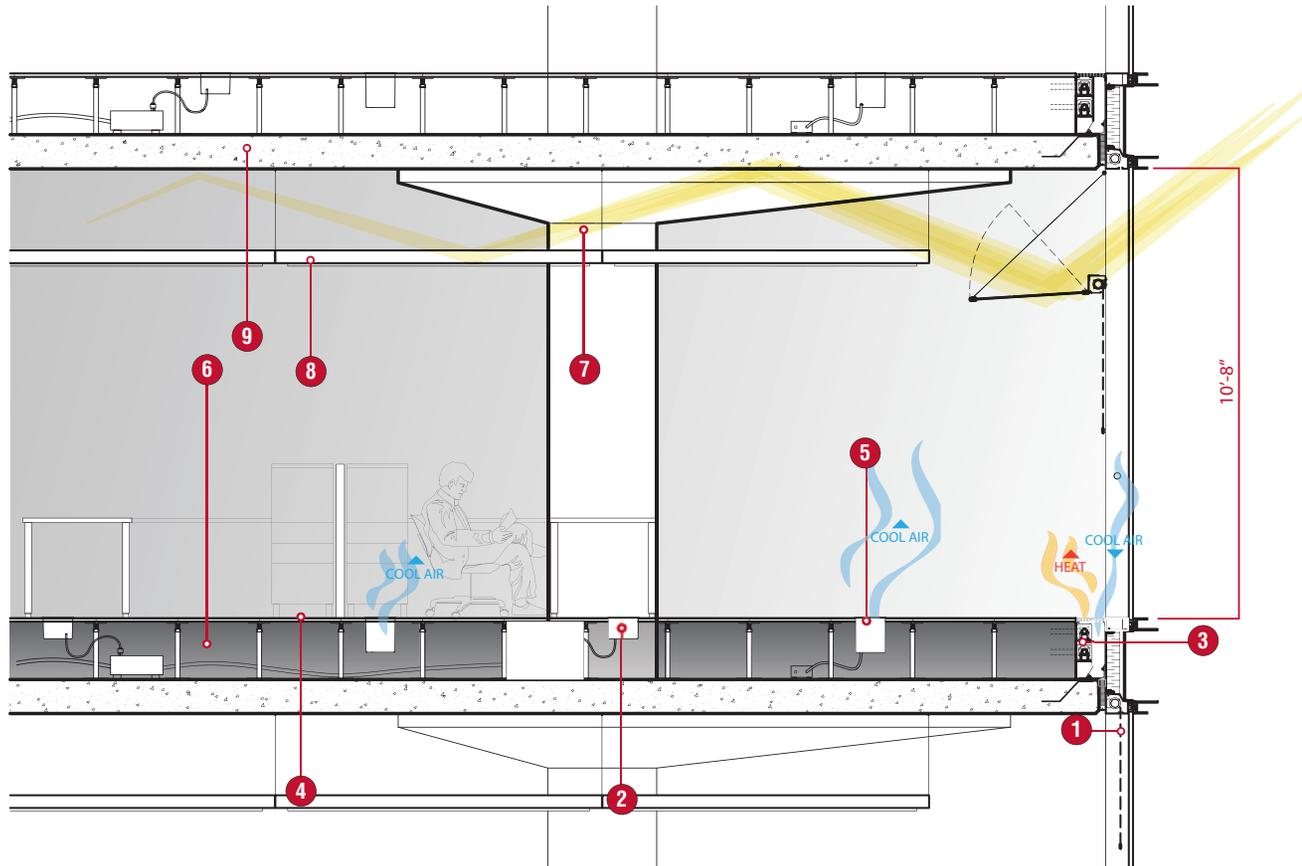
**1. WINDOW SHADING:** Interior roller blinds at all glazed walls. Exterior horizontal aluminum fin type sun shading at the south facing façades. Exterior vertical sun shading at the west façade.
